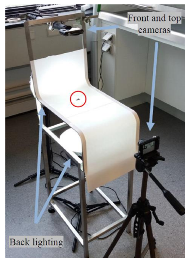
Figure 7-6: Camera setup with two cameras to determine particle size and shape.
