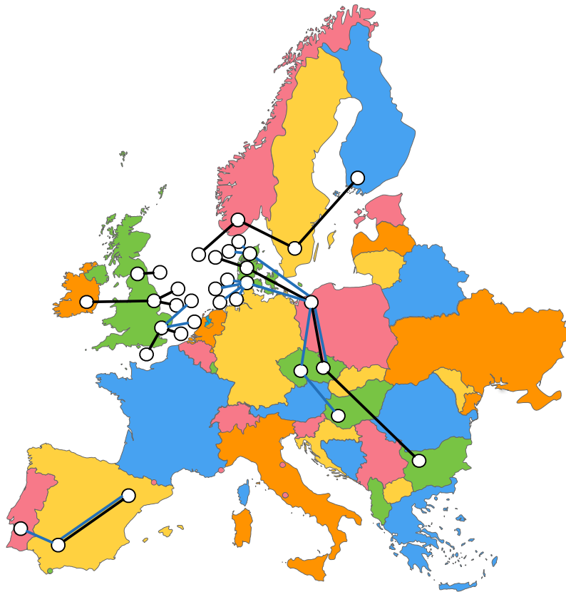
Figure 3.9: Step 2 of the DC upgrade scenario. Lines added in step 1 are marked in black, while lines added in step 2 are marked in blue. Source: [Pub. G] .
