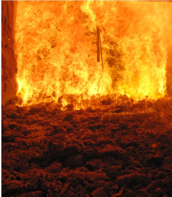
Figure 5.6: Picture of the combustion of waste on a grate at Affald+ during the measurements in this study. The probe is measuring in measuring point 4 during plant setting 2. The tip of the probe is outside of the flame region; the devolatilisation zone.
