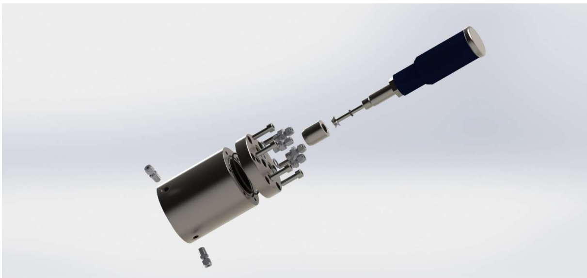
Figure A-4 3D sketch of the Equilibration and Dilution Cells
