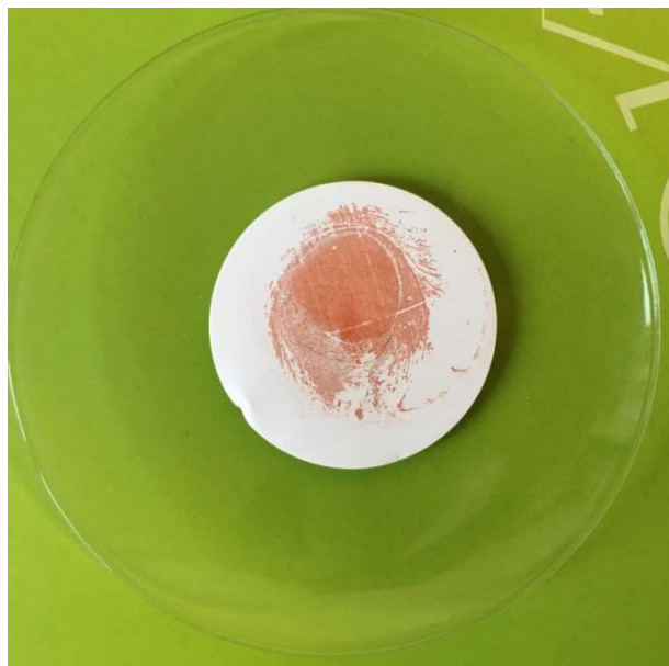
Figure 6.6 Change of color of \text{FeCO}_3 after solubility analysis
