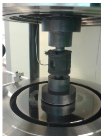
Figure 2.2: Graphite die with powder mounted in SPS system.
