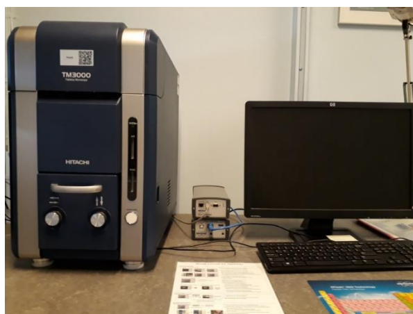
Figure 2.8: TM3000 tabletop scanning electron microscope with energy dispersive x-ray spectrometer.
