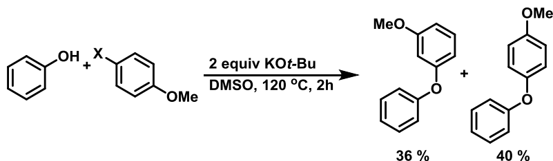
Scheme 29: Metal and ligand free Ullmann reaction by Yang et al. 97
