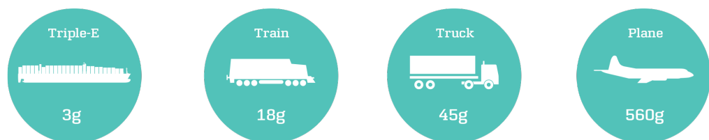
Fig. 1 Grams of CO 2 emitted by transporting 1 tonne of cargo 1 km, using respectively container vessels, trains, trucks or planes. (Source: Maersk, 2015)
