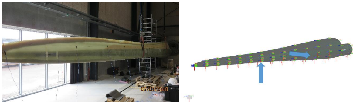
Figure 3 Instrumented blade on the test stand in the free-free support configuration (left) and geometry of the measurement and excitation points (right).
