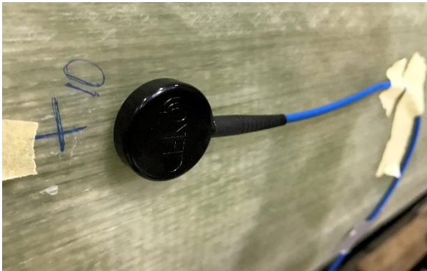
Figure 12 The optical accelerometer (CEKO OA1) was mounted flap-wise on the test blade. The accelerometer measures 27 mm in diameter. The first 7 resonance frequencies measured using the optical accelerometer and a reference piezoelectric accelerometer are shown in the table.
