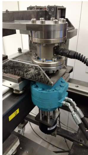
Figure 4.6. Sequential arrangement of TLC, actuator and ADT on the carriage plate.
