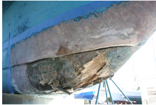
(a) Keel damage due to grounding ( picture courtesy, Sailor's Wharf, FL ).
