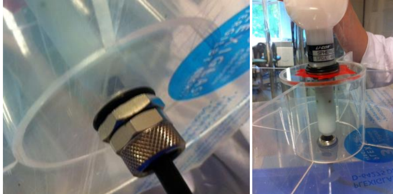
Figure S3: The fitting on the bottom of the reactor, used to mount the cable of the light sensor (picture on the left). The plastic fitting, used to keep the light sensor in a vertical upward position inside the reactor (picture on the right).
