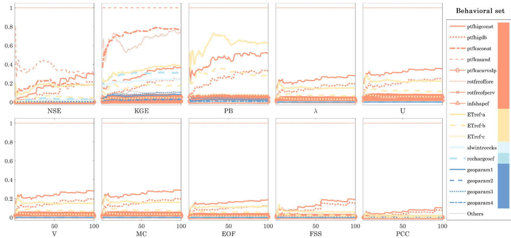
Figure 3. Average accumulated relative parameter sensitivities over 100 behavioral (NSE > 0.5) initial parameter sets and one-at-a-time parameter perturbations. The different colors indicate different model processes. The red coded parameters refer to soil moisture, yellow to evapotranspiration, ice blue to interflow, light blue to percolation, and dark blue to geology.
