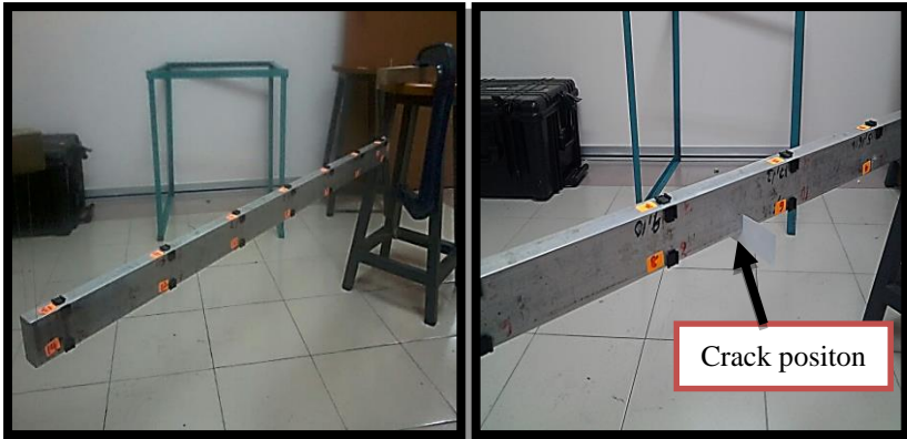
Figure 2: Aluminum beam is suspended with soft string to support the beam in free-free condition and the crack position is indicated
