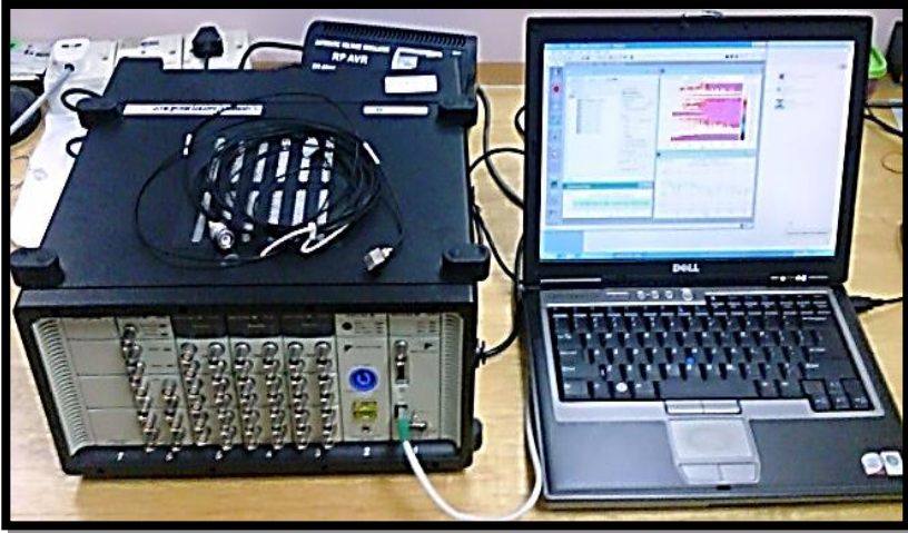
Figure 1: The Bruel&Kjaer PULSE™ Multi-Analyzer System connect to a computer with MTC™ software and Operational Modal AnalysisPro™ software.
