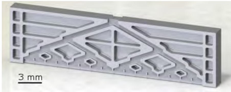
Figure 6.1: CAD model of the microfluidic dispenser which was used as study case for the simulation-assisted part design, captured in SolidWorks®. Shown is the front part, the back looked exactly the same because of the part symmetry.
