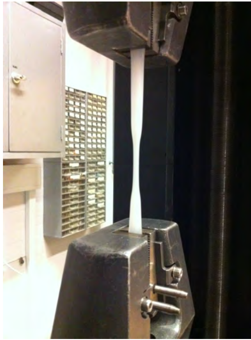
(a) PP specimen in machine during test.
