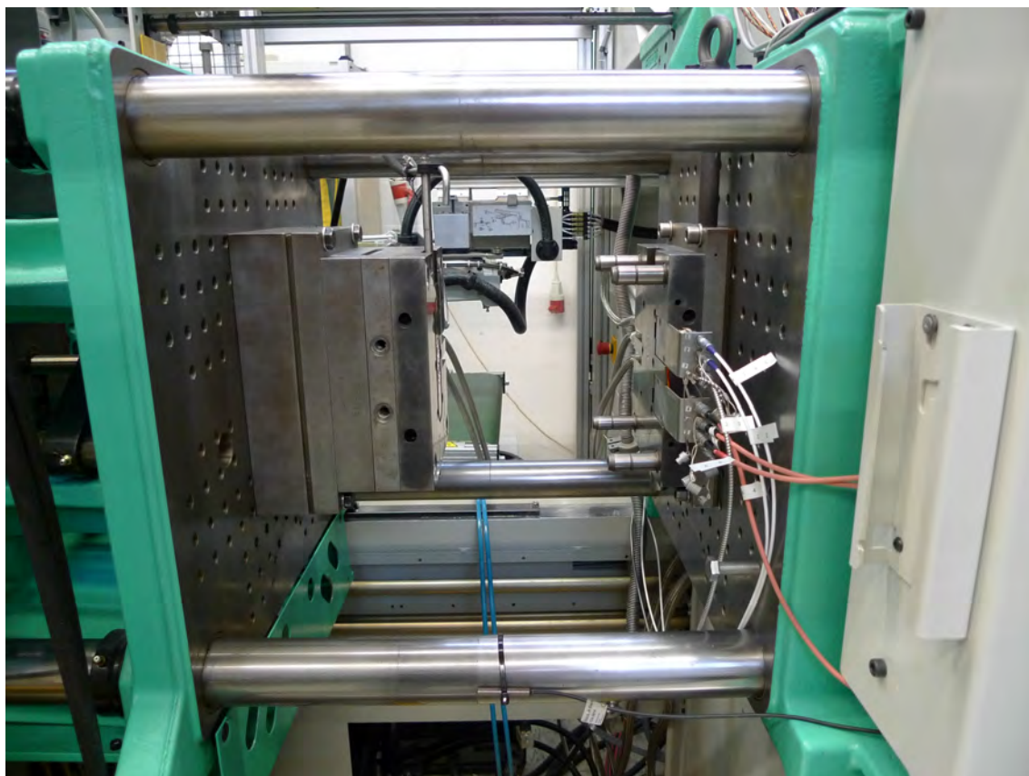
Figure E.2: Mold installed on the injection molding machine.
