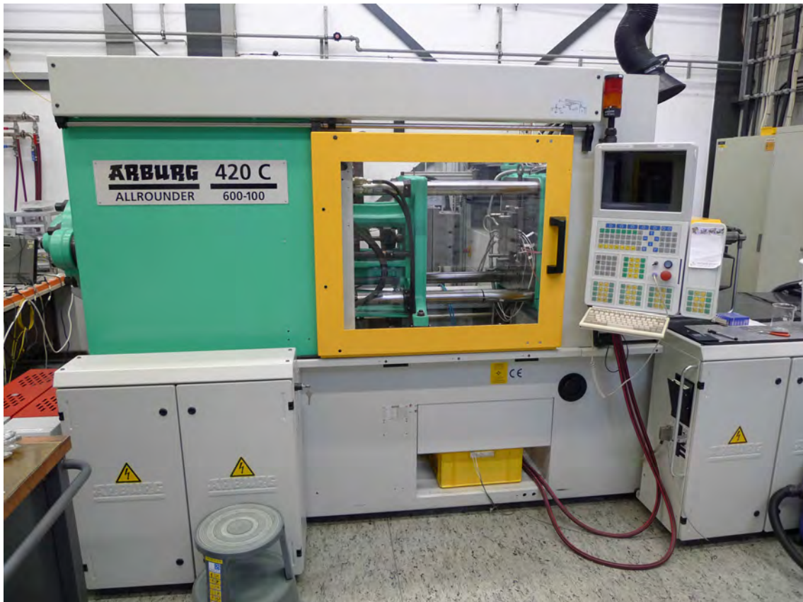
Figure E.1: Arburg Allrounder 420 C 600-100 injection molding machine.
