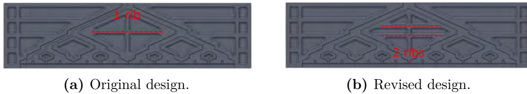
Figure 6.9: Design optimization at the microfluidic dispenser. It was equipped with one more rib for more uniform flow on both sides.
