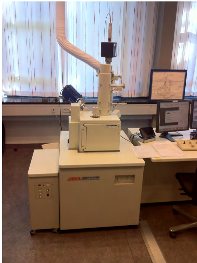
Figure C.2: JEOL JSM-5900 scanning electron microscope.
