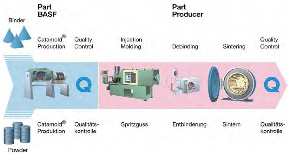
Figure 2.3: Schematic of the typical process chain of powder injection molding. Optional finishing processes like polishing, plating, or grinding after sintering are not shown. The blue part (left) is usually covered by the material supplier, the pink part (right) is covered by the component manufacturer. [22]
