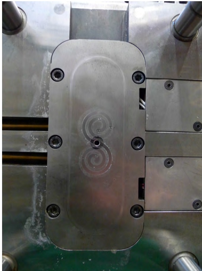
Figure E.3: Stationary half of the double test spiral geometry with sprue and pressure sensors.
