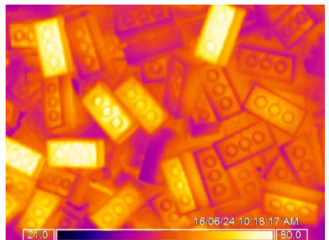
Fig. 7. Thermographic image of the produced parts indicating temperatures ranging from 21 to 80°C.
