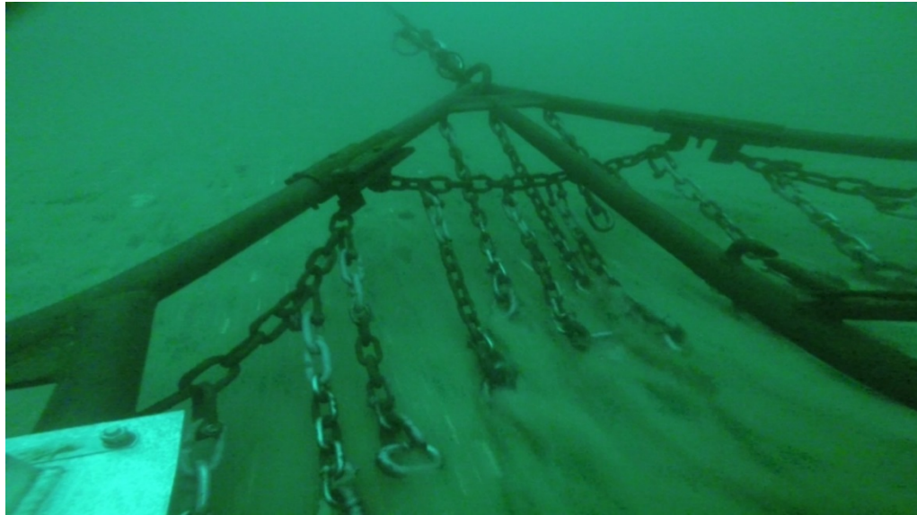
Figure 12.123.1: Still images from GoPro camera attached to dredge frame. Tickler chains making bottom contact during comparison tows.
