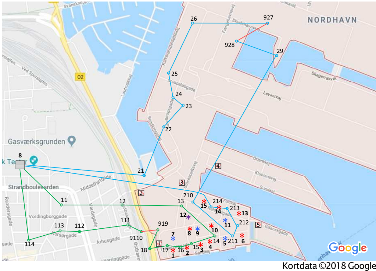
Fig. 4: Nordhavn city district. Electrical network: green and light blue lines - electrical distribution system layout (simplified), red lines - tie-lines between feeders; gray rectangle (8) - main substation, circles - secondary substations 10/0.4 kV. Heat network: the asterisk * - heat customer, purple * - group of single houses, red * - apartment block, blue * - office building; shaded square - possible location of HP
