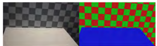
Fig. 6. Labeling of the image to the left results in the label image to the right. Each color in the label image represents a label that we assign a BRDF to. The black edges between labels indicate areas where we apply a nearest neighbor method.
