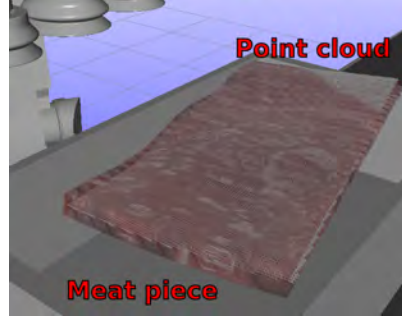
Fig. 15: The simulation of the grey point cloud is done using RobWork [37]. The meat piece is transparent such that the entire point cloud can be seen. Furthermore, the point cloud is slightly translated and rotated to model the effect of uncertainties in the vision system.
