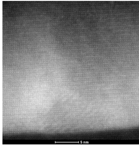
Figure 2.8 HAADF-STEM image of GBCO film grown on SrTiO 3 (001) substrate.
