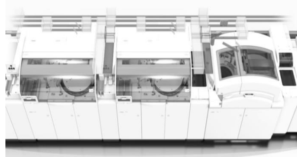
Figure 2. Automated laboratory [52] with internal transportation system based on conveyor belts
