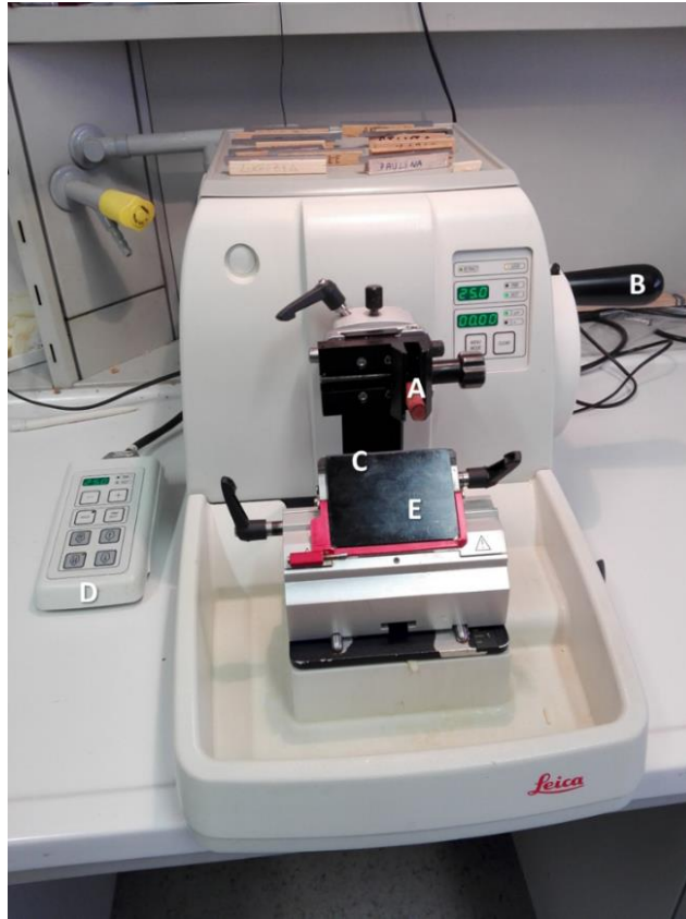
Figure 2.1: Rotary microtome Leica RM 2245 (Leica Biosystems, Nussloch, Germany). The debarked sample (A), by rotating the handle (B), is cut in micro-sections by the blade (C) at a pre-determined thickness (D) and collected from the designated surface (E).
