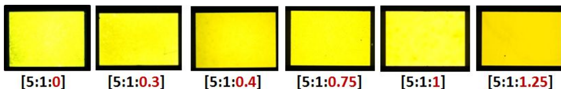
Figure 6.15 Photographs of DNA-CTMA based LEC under operation. Each pixel corresponds different salt content in the blend of SY:DNA-CTMA-TBABF 4 [5:1:.x].
