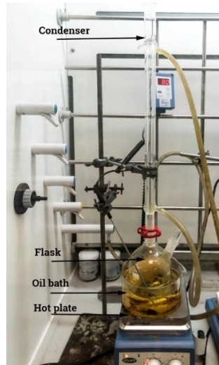
Figure 6-5: Set up used to measure the constituent content of carbon fibre composite laminate.
