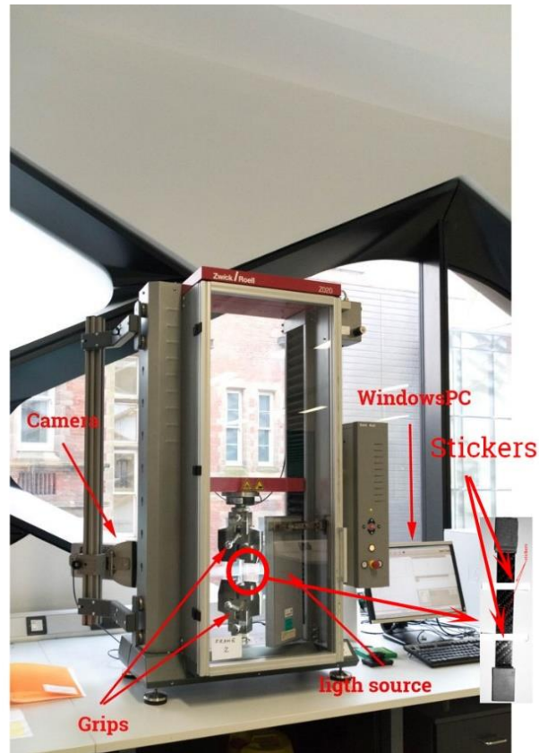
Figure 6-3: View of tensile test frame, Zwick/Roell Z020.
