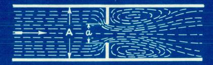
Fig. 2.1 Section through a parallel pipe shewing the acceleration of the fluid stream through an orifice.
