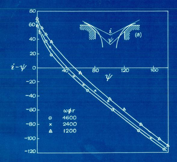
Fig. 14.6 The relationship between the curvature of the flow lines and the orifice champfer.
