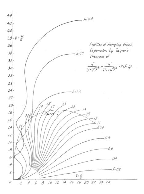
Fig. 20.1. Profile of Hanging Drops (calculated by Freud and Herkins)
