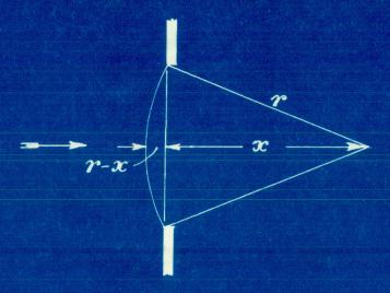
Fig. 2.4 Diagrammatic representation of an equi-velocity spherical-cap surface.
