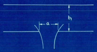
Fig. 9.3 Dimensions of an orifice in the wall of a pipe.
