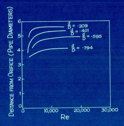
Fig. 17.2 The position of the maximum pressure recovery.
