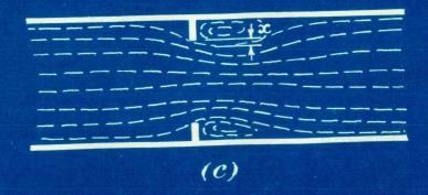
Fig. 2.3 Pictorial representation of the effect of the orifice-diameter ratio on the coefficient of contraction.
