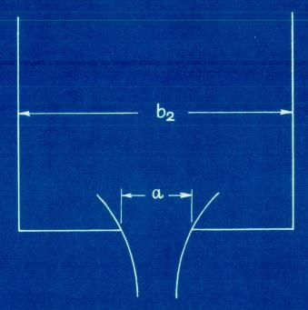
Fig. 9.4 Dimensions of an orifice in the end of a pipe.
