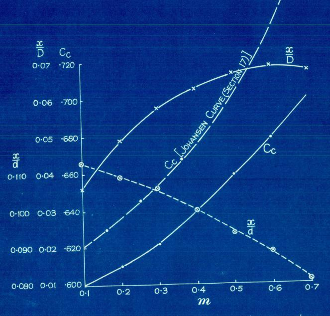
Fig. 2.2 The effect of the orifice-pipe diameter ratio on the coefficient of contraction. Values given by WITTE(2)
