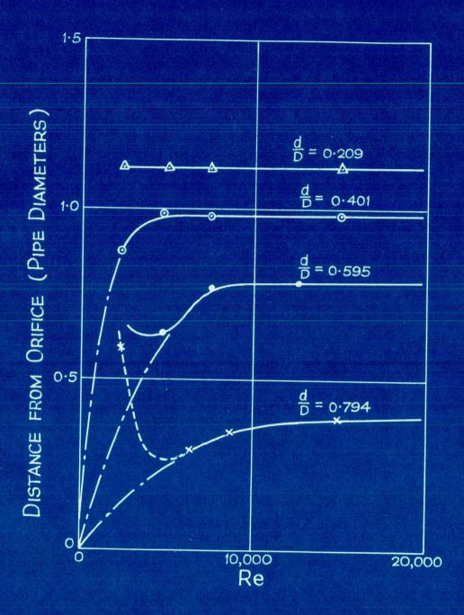
Fig. 16.1 Position of the downstream minimum pressure.
