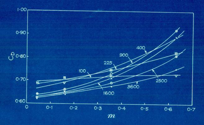
Fig. 11.2 The variation of CD with "m" for various Reynolds Numbers (TRANSITION ZONE)
