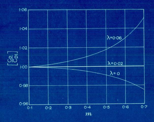
Fig. 9.5 The effect of a pipe roughness on orifice discharge
