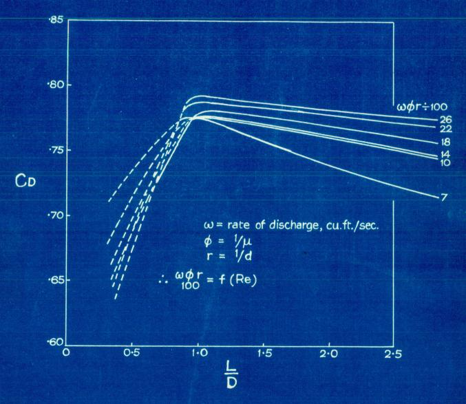
Fig. 13.1 The variation of CD and  $\frac{L}{D}$  at various values of Re. (Zuckrow)
