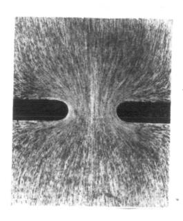
Fig.5.1. Flow through a rounded orifice.
