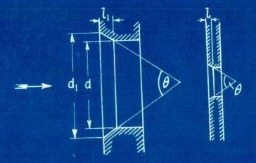
Fig. 3.1 (b) Geometrical similarity of a champfered orifice.
