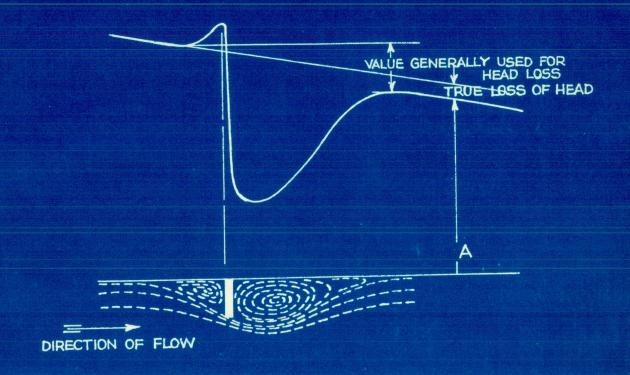
Fig. 17.3 Illustration of the correct measurement of head-loss due to an orifice.
