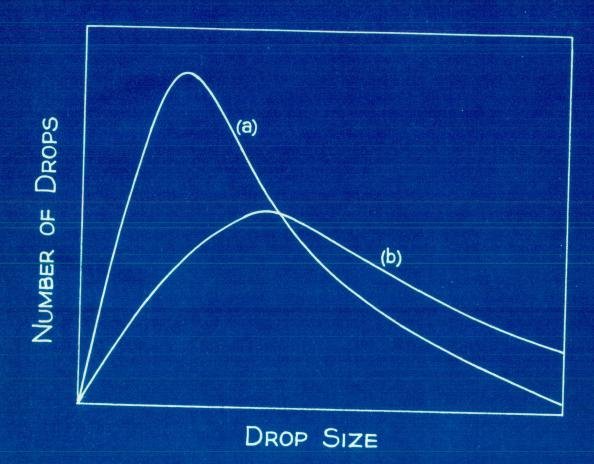
Fig. 24.1 Frequency curves measuring the atomisation of a spray.
