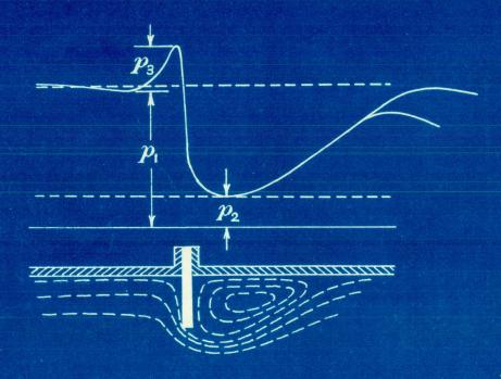
Fig. 2.5 The pressure distribution across a thin orifice plate.
