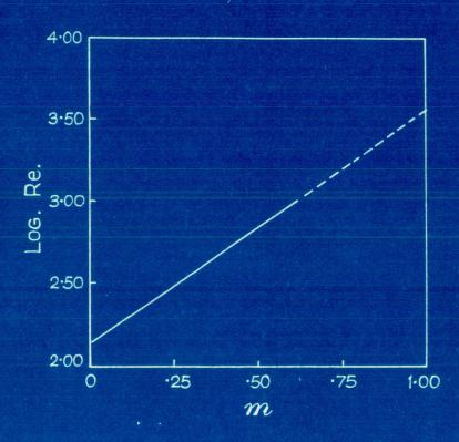
Fig. 5.4 The variation of Reynolds Number for maximum discharge coefficient with the orifice ratio.
