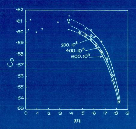
Fig. 11.1 The variation of C<sub>D</sub> with "m" for various Reynolds Numbers (TURBULENT ZONE)
