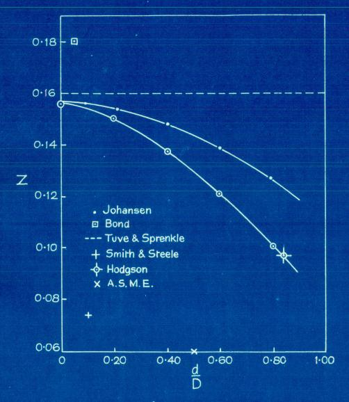
Fig. 5.3 The effect of orifice size on the viscous discharge.
