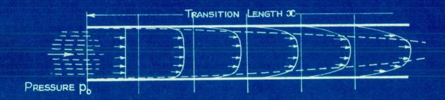
Fig. 9.1 The development of the velocity profile in the "inlet length" of a pipe.
