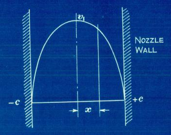
Fig. 2.6 Velocity distribution across the wall of a nozzle.
