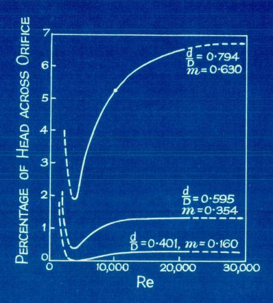
Fig. 15.3 The variation of orifice pressure-rise with Re and m
