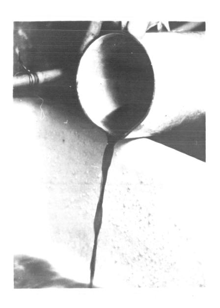
Fig. 21.1. Stationary Waves of a jet. (Obtained by Author).
