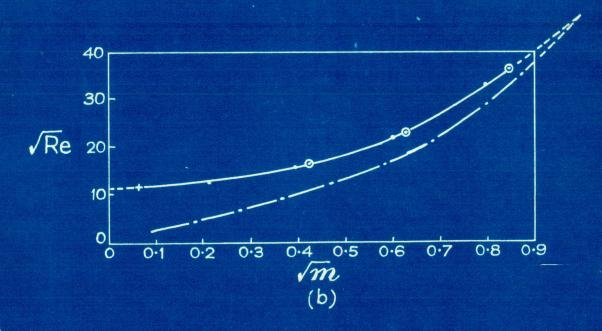
Fig. 11.3. The Maximum Discharge Coefficient and Limiting Reynolds Number.
