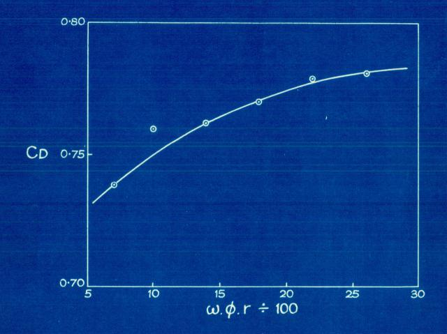
Fig. 13.2 The effect of Re on the CD of a mouthpiece  $\frac{1}{\alpha} = 2.0$ .
