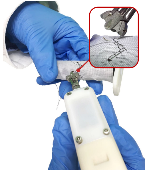
Fig. 1. Sewing a Stent Graft with the Proposed Device
