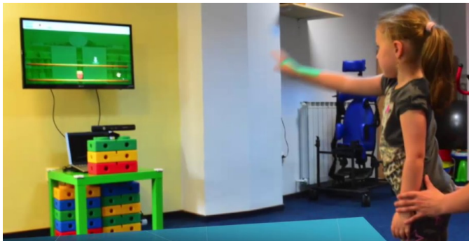
Fig. 1: MIRA system including a Kinect sensor to detect user’s motion and software to match an exercise with a game.
