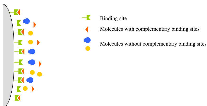
FIGURE 1.11: Mechanism of affinity chromatography
