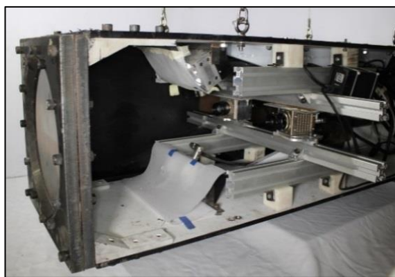
Fig. 7- Photograph showing the inside of the modified, DIC pendulum, set up for filming the rear surface of the plates
