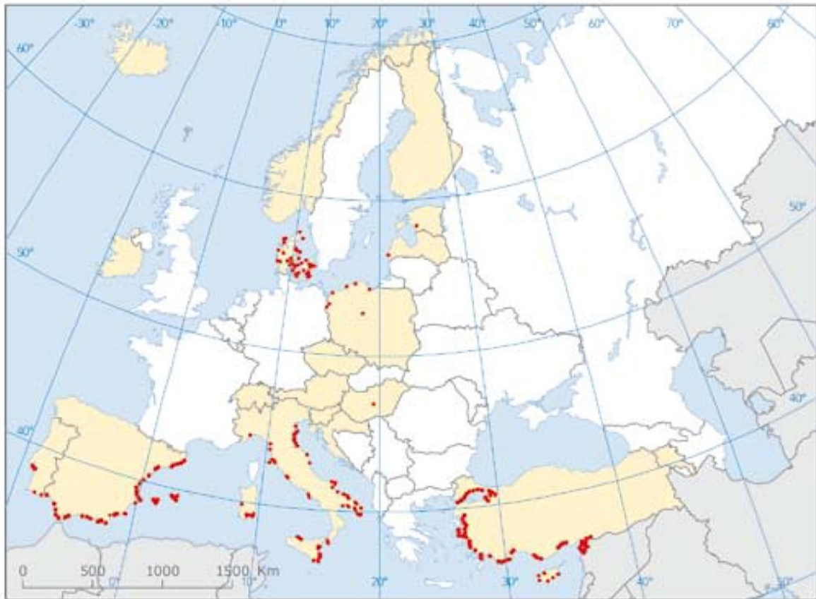
Figure 1.1: a) coastal areas vulnerable to saline intrusion in continental United States (adapted from Sawyer et al. (2016)) and b) recorded incidences of seawater intrusion in parts of continental Europe (EEA, 1999).
