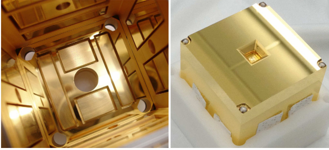
FIG. 2. Left: A view up into the sensor housing, centered on the upper z -face. The test mass and lower z -face have yet to be integrated and the ISUK entry points are just out of shot. The two x -faces are on the left and right of the image while the y -faces can be seen at the top and bottom. The empty recesses where four of the caging fingers enter can be seen in the corners and the plunger entry hole can be seen in the center. The electrodes set within the walls are clearly visible. Right: One of the flight test masses with the lower half temporarily held in a protective case. Note the caging corner domes with the underlying gold-platinum surface exposed. Credit: OHB Italia SpA.
