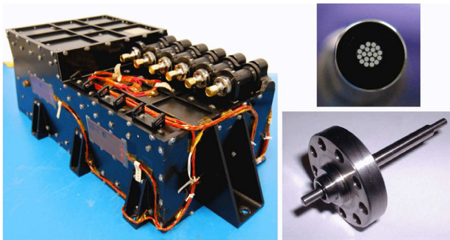
FIG. 1. Left: The flight ULU with external heaters attached. The ends of the six optics barrels are seen temporarily sealed with gold dust caps. Top right: An end-on view of an FOH with the 19 individual cores visible. Bottom right: A flight ISUK.
