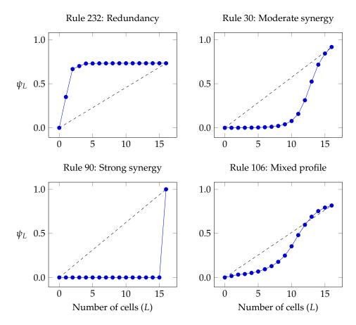
**Figure 4.** While the concave shape of  $\psi_L$  for Rule 232 shows that correlations are mostly redundant, the convex shape for Rule 30 shows the dominance of synergies of order 10 or more. Rules 60 and 90 are the only rules that generate purely synergistic structure of the highest order. Results for Rule 106 show an inflection point where  $\psi_L$  switches from convex to concave, suggesting the coexistence of synergistic small-scale and redundant large-scale structures.
