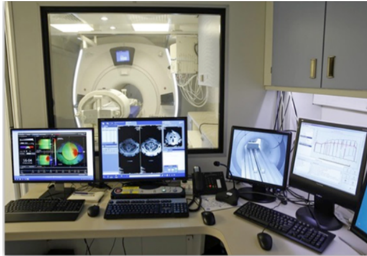
Figure 4 MRI hyperthermia suite in the Erasmus Medical Centre (Rotterdam, Netherlands) consisting of the control and MRI rooms equipped with the BSD-2000 hyperthermia system (Pyrexar Medical); Illustration of the treatment control through the SigmaVision®Advanced software (Dr. Sennewald Medizintechnik), (image by kind permission from Pyrexar Medical and Dr. Sennewald Medizintechnik).
