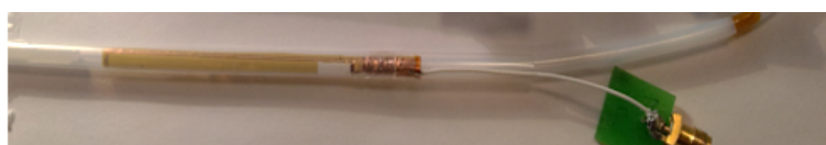
Figure 5 Somatex laser applicator integrated with a micro-coil for operation at 3T.
