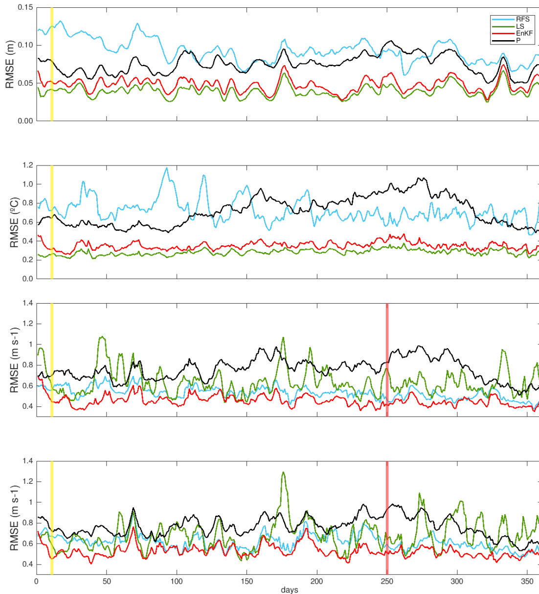
Figure 3.4: RMSE time series (from January 1 st , 2010) of the validation with respect to GHRSSST, AVISO altimetry, and Globcurrent datasets to validate (from top to bottom): SST, SSH, U, and V. Blue corresponds to the reconstructed full-space state (RFS), green is the Least Squares (LS) solution, red represents the ensemble-mean (analysis) after the EnKF was applied using the NN, and black is the analysis using the EnKF and persistence (P). Yellow and pink shades are centered on the snapshot days in Fig. 3.9 and 3.8.
