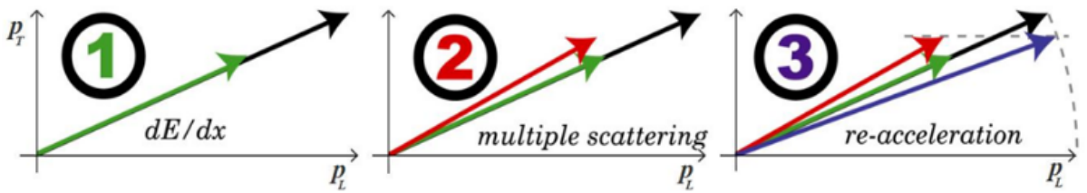
Figure 2.2: A visual representation of Equation 2.74. The black arrow characterises the muon’s momentum as it enters the absorber. As the muon traverse the absorber material it loses energy in all directions, shrinking in momentum space. The resulting muon momentum is now represented by green arrow in plot (1). Multiple scattering within the material may then cause heating effects and must be limited as this could increase the formerly reduced (green arrow) transverse momentum (2). The third plot signifies the desired case within MICE when the muon beam subsequently reaccelerated longitudinally such that 4D transverse beam cooling is observed. The blue arrow then represents the end results in 2D [138].
