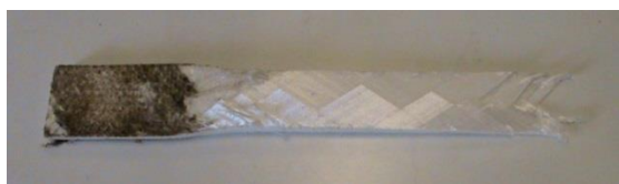
204 205 Figure 10. Failure of tension shear specimen.
