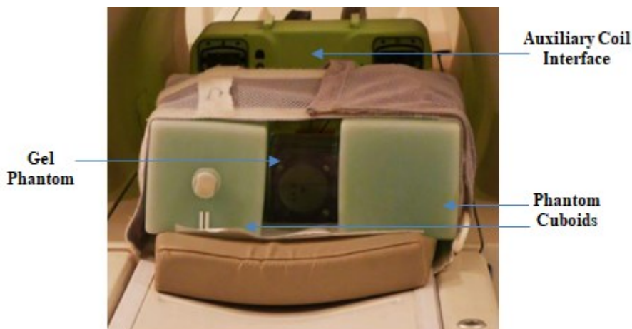
Figure 6.24 Arrangement for MRI scanning of directly-coupled system.
