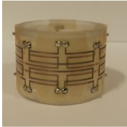
Figure 4.36 Final coupled MI ring device with L_v = 4 mm, L_h = 24 mm, diameter = 34 mm, length = 18 mm
