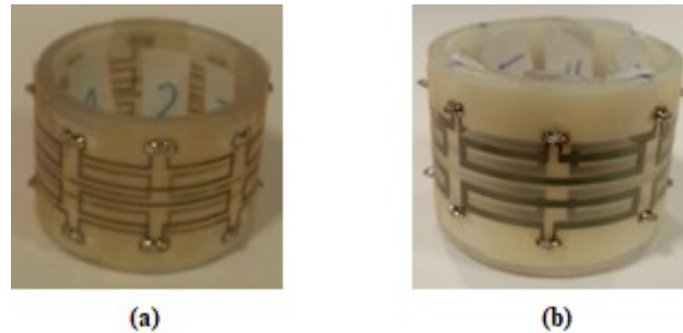
Figure 4.41 Coupled MI ring devices with track widths of (a) 0.35 mm and (b) 1 mm.
