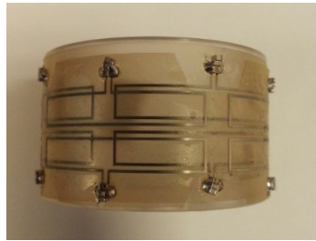
Figure 4.44 Larger coupled MI ring device: diameter = 49.5 mm, length = 22 mm, L_v = 6 mm, L_h = 35 mm.
