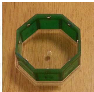
Figure 1.32 Magneto-inductive ring made from 8 inductively coupled loops 4 .
