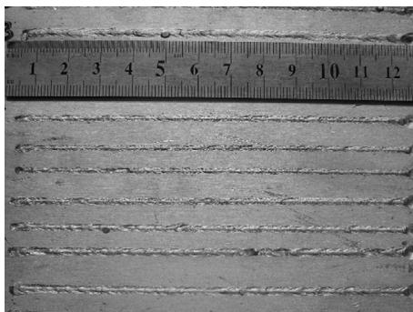
Fig. 2. Autogenous bead on a plate welded AA2024-T3 of different welding speeds.
