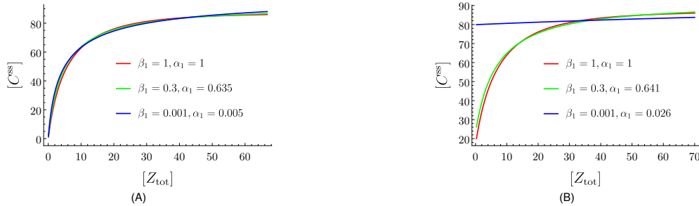
FIGURE 3.9: Evidence that accidental leak reactions limit the degree to which coupling between \mathcal{U} and \mathcal{I} can be reduced whilst maintaining a functioning network. (A) In the absence of a leak reaction, one can decrease \alpha_1 and \beta_1 successively using exactly the procedure outlined in Section 3.5, maintaining an approximately constant input-output curve. (B) In the presence of a leak reaction caused by a signal molecule Z' , one is able to reduce \alpha_1 and \beta_1 to match a given input-output curve whilst the coupling of Z' remains relatively weak. However, eventually Z' becomes dominant and one cannot find suitable parameters \alpha_1 and \beta_1 to match a given input-output curve well. Parameters used for both networks: [X_{\text{tot}}] = 150 , [Y_{\text{tot}}] = 100 , [Z'_{\text{tot}}] = 100 , [P_{\text{tot}}] = 100 , \alpha_1 = \beta_1 = 1 , \alpha_2 = \beta_2 = 10 , \gamma_1 = 0.01 , \gamma_2 = k_1 = k_2 = k_{\text{on}} = k_{\text{off}} = 10 , k_3 = 1 .
