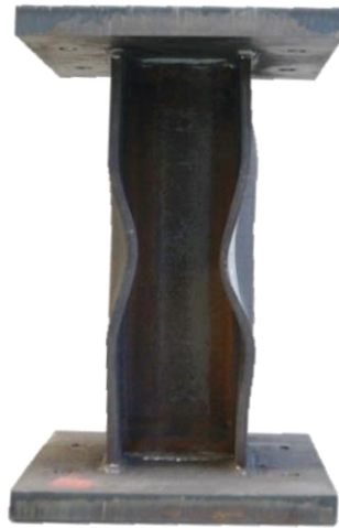
Fig. 7. Typical failure mode of stub columns (B7)
