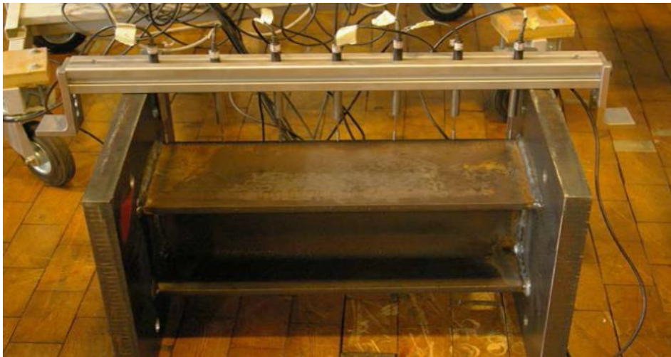
Fig. 4. Test setup for geometric imperfection measurements
