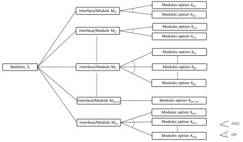
Figure 4 AND-OR Tree diagram for modelling different OPAP Configuration
