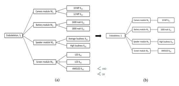
Figure 6 (a) AND-OR tree diagram for OPAP smartphone with different module options (b) A feasible product configuration for OPAP smartphone
