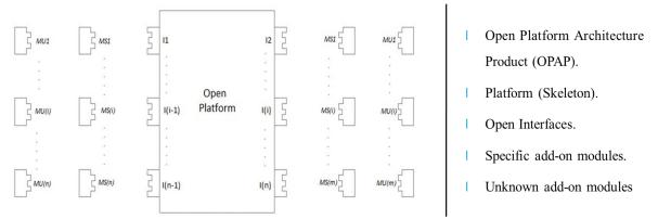
Figure 2 Schematic representation of an OPAP with platform, interfaces and module options
