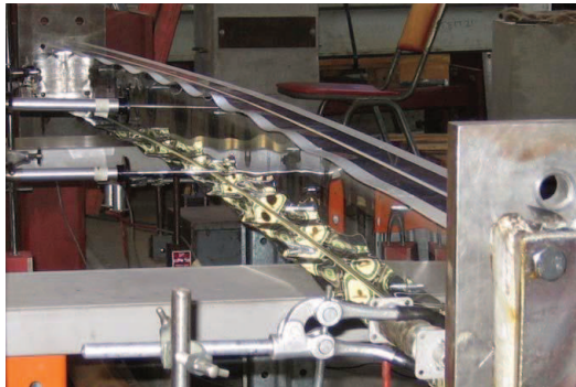
Figure 2.18: Interactive buckling observed in a stainless steel I-section strut (Becque, 2008).
