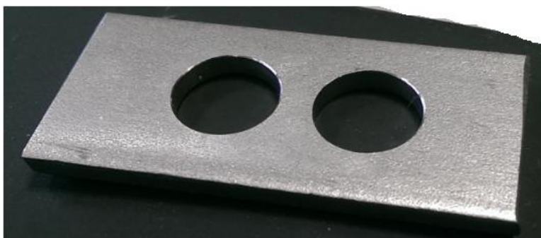
Figure 2.2. Coupon mould designed to allow compression of CDC coupons. Dimensions 3.2mm thick, holes are 13.00mm in diameter.
