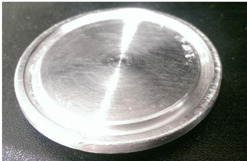
Figure 1.31. 316 stainless steel inlet/outlet blank sample of used manufacturing plant, taken from a well-used 100L vessel.
