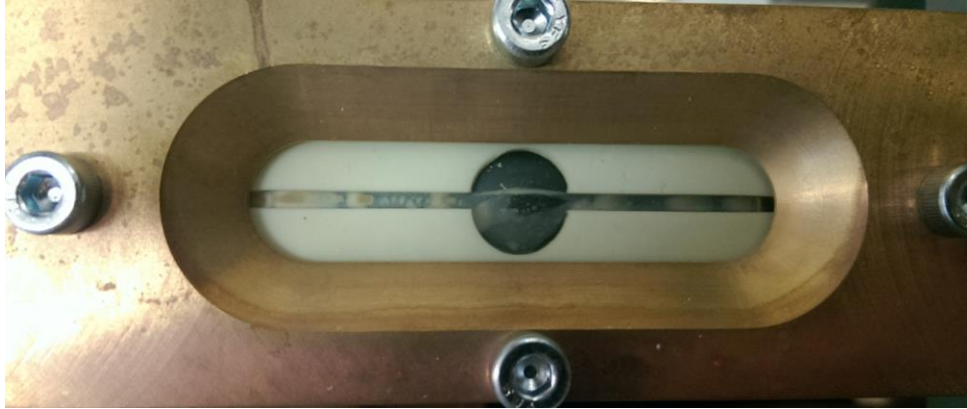
Figure 3.16. Picture of a smooth 304 stainless steel substratum with PA01 cultured for 2 days in AB minimum growth medium at room temperature. Points of interest are the microbes appearing to be growing well in the inlet and outlet area of the flow cell.
