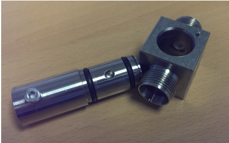
Figure 3.5 – ½” Stainless steel feeder with drilled cup and valve body.
