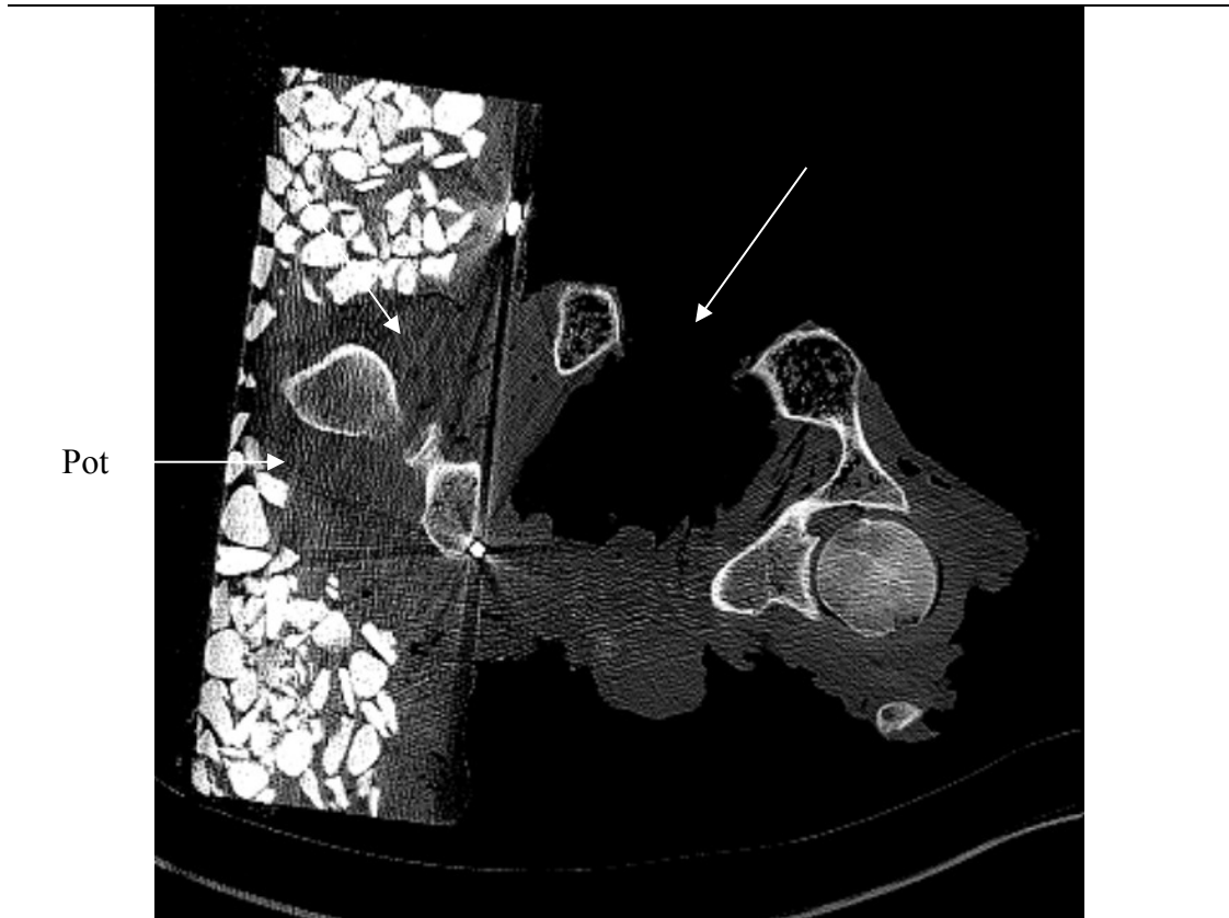
Figure 7.32: Axial CT scan of Test 5 demonstrating the pubic symphysis opening (arrow).
