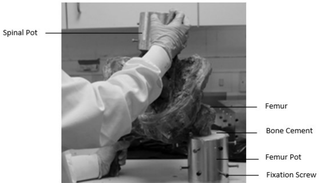
Figure 7.13: Photograph of the potting. The specimen is held in an upright position with the femur placed in its pot while the bone cement hardens.
