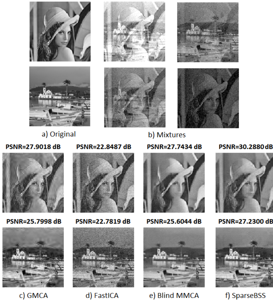
Figure 3.5.5: Two classic images, Lena and Boat were selected as the source images, which are shown in (a). The mixtures are shown in (b). The separation results are shown in (c)-(f). We compared SparseBSS with other benchmark algorithms: FastICA [42], GMCA [10] and BMMCA [3]. We set the overlap percentage equal to 50% for both BMMCA and SparseBSS. The recovered source images by the SparseBSS tend to be less blurred as compared to the other three algorithms.
