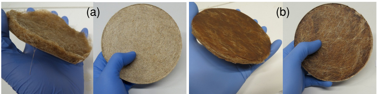
Figure 6.8 Nonwoven flax fiber preform before and after hot pressing (a) non-woven flax preform without any binder, (b) non-woven flax preform containing 10% ABW nanofibers as binder.
