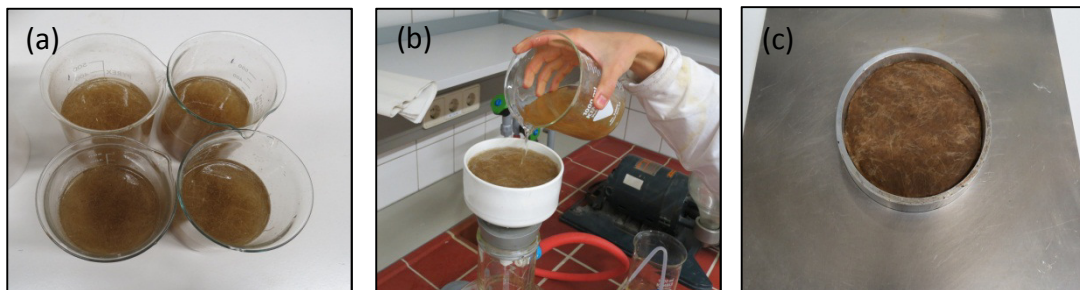
Figure 3.5 Preparation of ABW/Flax preform: (a) flax fiber soaked in ABW suspension overnight, (b) filtration of ABW/Flax mixture, (c) ABW/Flax preform in mold before hot press.
