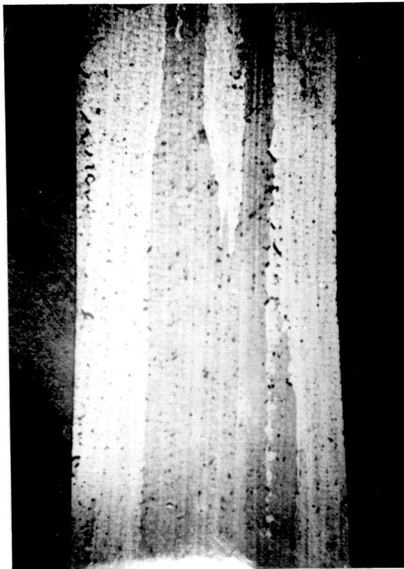
Figure 4.12: Longitudinal section of test N25 showing double neck
