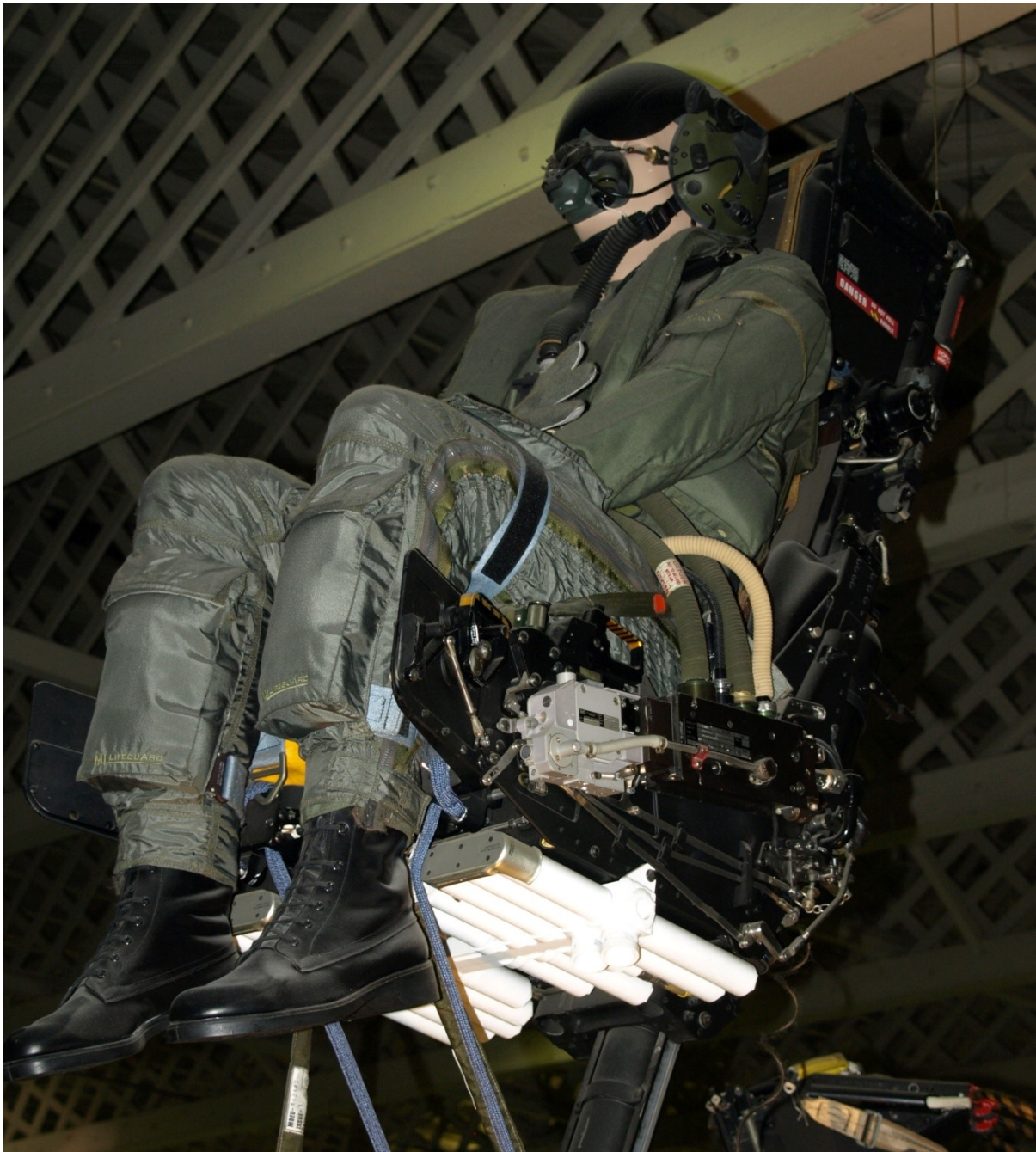
Figure 37: Martin Baker Mk 10 ejection seat. Note the white rocket packs under the seat. Taken from [134]
