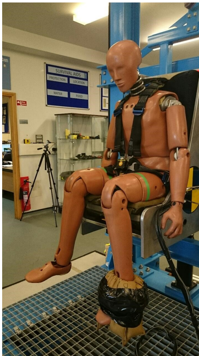
Figure 13: Hybrid III anthropometric test device on a drop tower. The simple cervical spine is clearly visible. Author's photograph.
