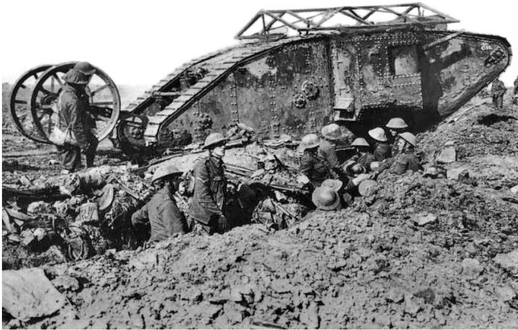
Figure 10: British Mark 1 tank on the Somme. Note the wire mesh to protect against dropped hand grenades. Copyright expired image [70].
