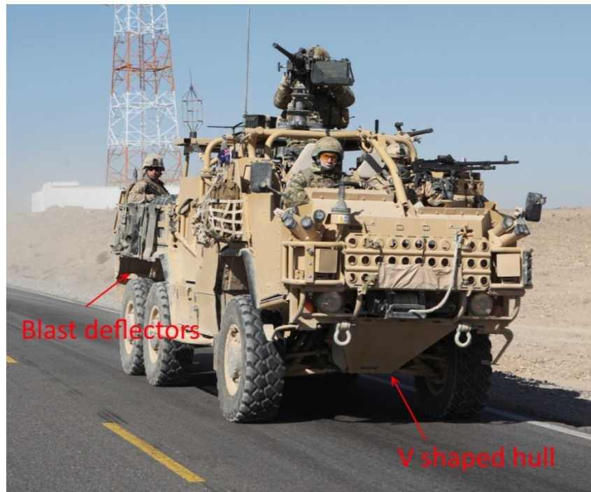
Figure 11: Coyote vehicle in Afghanistan. Note the V shaped hull, high ground clearance, and blast deflectors, all designed to reduce the effect of underbody blast. Public domain image [40].
