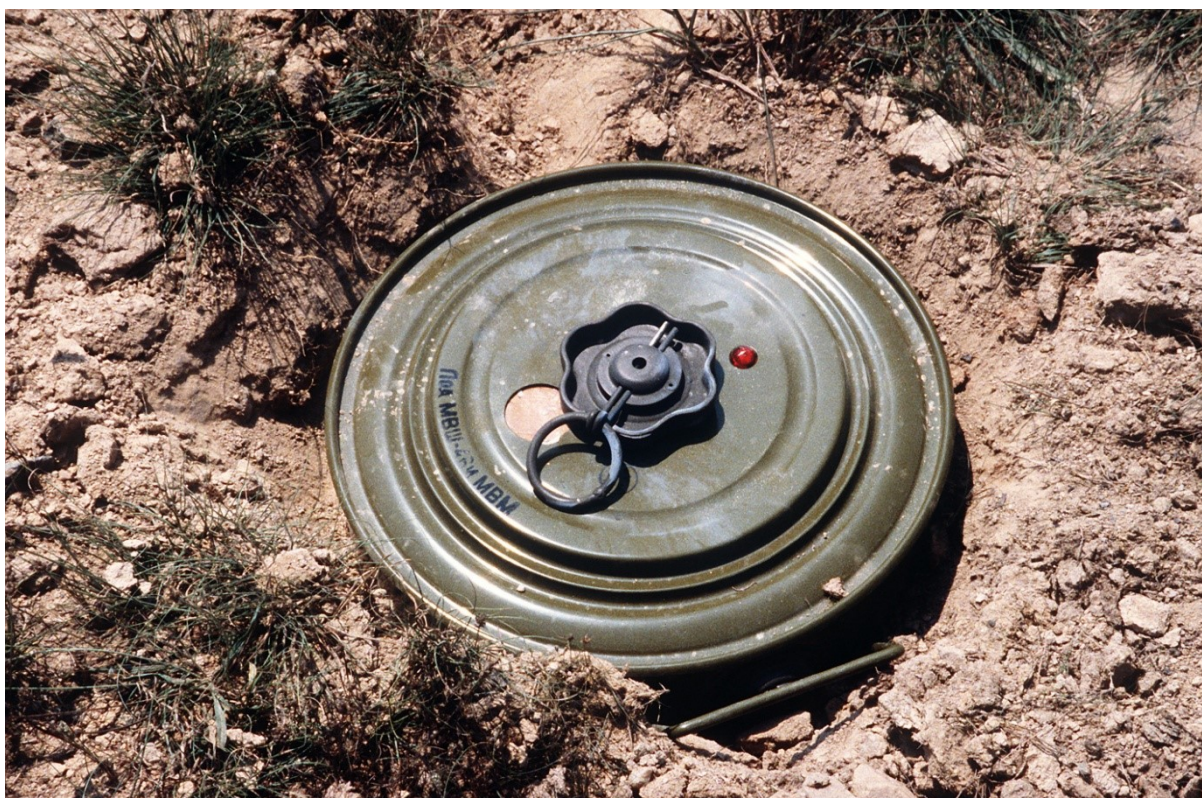
Figure 3: Anti tank mine, with a large upper surface and a trigger designed not to be fired by a pedestrian. This device is a blast weapon [3].
