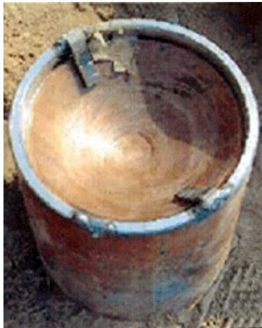
Figure 4: Explosively formed penetrator. Note the copper dish on top of the device which forms the penetrator [7].
