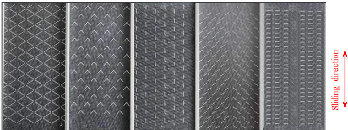
FIGURE 3.29: Pocketed fused silica test pads employed in the first stage of the research.
