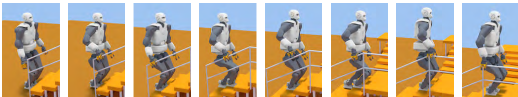
Figure 4.12: Snapshots of the climbing 15-cm high steps motion with handrail by the TALOS robot in simulation.
