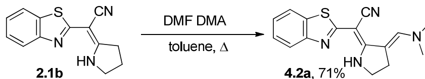
Scheme 4.1. Formylation reaction of enaminonitrile 2.1b with DMF DMA.
